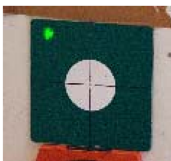
Figure 2: Photograph of a Cyra target with the green laser dot in the top left hand corner.
